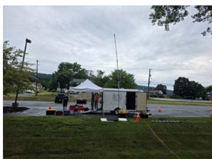
View from the generator (yellow power cord on the right) showing the new collapsible pole supporting the Carolina Windom antenna.
