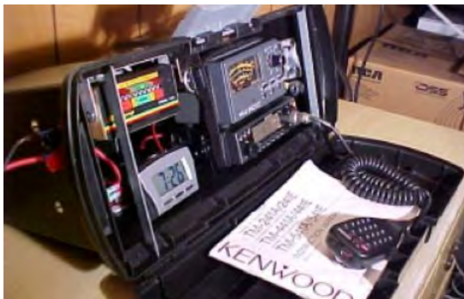
This Go Kit is in one of those plastic tool boxes. Note the external connections for power.
